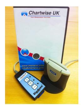
The Depot Downloading – Ideal for a transport office this package includes the Digidown, a driver card reader which can be placed in the transport office and software which allows simple visualisation of driver card data. This means the transport manager can see at a glance the activity of each driver. For operators with multiple sites, multiple depot downloading systems will be required.
